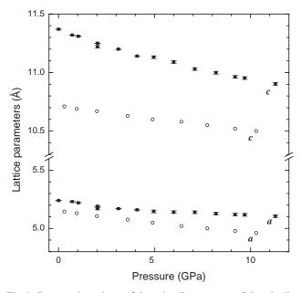
Fig. 3. Pressure dependence of the unit cell parameters of the scheelite structure in  $CaWO_4$  and  $YLiF_4$ . Data for  $YLiF_4$  ( $\bigcirc$ ) are taken from Ref. [5] and data for  $CaWO_4$  are from the present study ( $\blacksquare$ ) and Ref. [8] ( $\blacksquare$ ).
