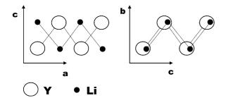
Fig. 9. Details of the scheelite structure (left) in the a-c plane with A (Y) and B (Li) cations located in alternate planes along the b-axis (perpendicular to the paper). Details of the M-fergusonite structure (right) in the c-b plane with A and B cations located in alternate planes along a-axis (perpendicular to the paper). The M-fergusonite structure derives from the scheelite structure when B cations shift along a-axis of the scheelite.
