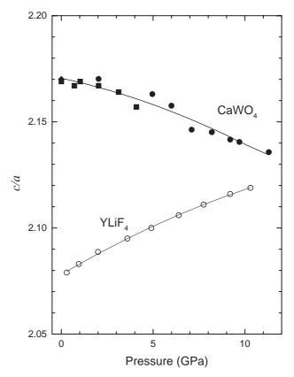
Fig. 4. Pressure dependence of the c/a ratio of the scheelite structure in CaWO<sub>4</sub> and YLiF<sub>4</sub>. Data for YLiF<sub>4</sub> ( $\bigcirc$ ) are taken from Ref. [5] and data for CaWO<sub>4</sub> are from the present study ( $\bullet$ ), Ref. [7] ( $\bullet$ ), and Ref. [8] ( $\blacksquare$ ). The lines are just a guide for the eye.
