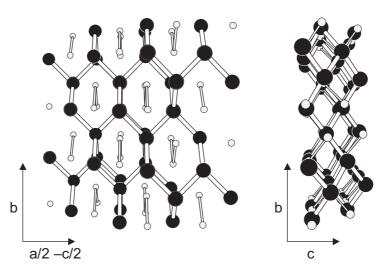
Fig. 7. Schematic views of the cationic arrangement in the M-fergusonite structure. The black atoms correspond to the A cation (Y), the gray atoms correspond to the B cation (Li). The anion atoms (F) are not shown for the sake of clarity. The shorter metal-metal distances are also shown.
