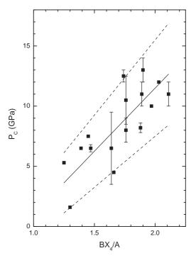
Fig. 10. Phase transition pressure in several scheelites as a function of the  $BX_4/A$  ratio. The symbols correspond to the data summarized in Table 1, the solid line corresponds to the relation given in Eq. (1), and the dashed lines indicate its lower and higher deviations.
