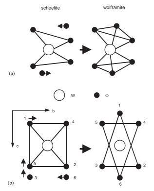
Fig. 8. (a) Schematic representation of the scheelite-to-wolframite model transition mechanism. (b) The (100) projection of a section of the scheelite structure compared to that of a portion of the wolframite structure. 1, 2, and 3 represent oxygen at (1/4,0,0) and 4, 5, and 6 oxygen at (-1/4,0,0).
