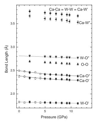
Fig. 5. Pressure dependence of the interatomic bonds in the scheelite structure of CaWO<sub>4</sub>. The solid lines show the pressure dependence of the Ca–O bonds and the dashed lines the pressure dependence of the W–O bonds. The solid symbols are from the present study and the empty symbols from Ref. [8].
