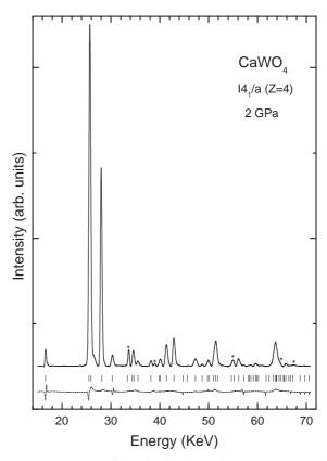
Fig. 2. EDXD pattern of the scheelite phase of  $CaWO_4$  at  $2\,GPa$ . The background was subtracted. The stars mark the position of the diffraction lines of the Au pressure marker. The last line represents the difference between the measured data and the refined profile. The bars indicate the calculated positions of the  $CaWO_4$  reflections.
