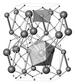
Fig. 1. Unit cell of the scheelite structure of  $ABX_4$  compounds with the a-, b- and c-axis. Big atoms refer to A cation (Ca, Y), the medium-sized atoms correspond to B cations (W, Li) and the small atoms to the X anion (O, F). Numbers 1 and 2 correspond to B-B distances of the diamond-like structure along b+c and a+c directions, respectively. The  $AX_8$  polyhedra and the  $BX_4$  tetrahedra are shown.
